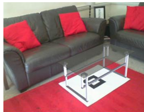
Figure 3: View showing virtual model (as through the viewing interface). The couches and room setting are real; the table a 3D CAD model.
